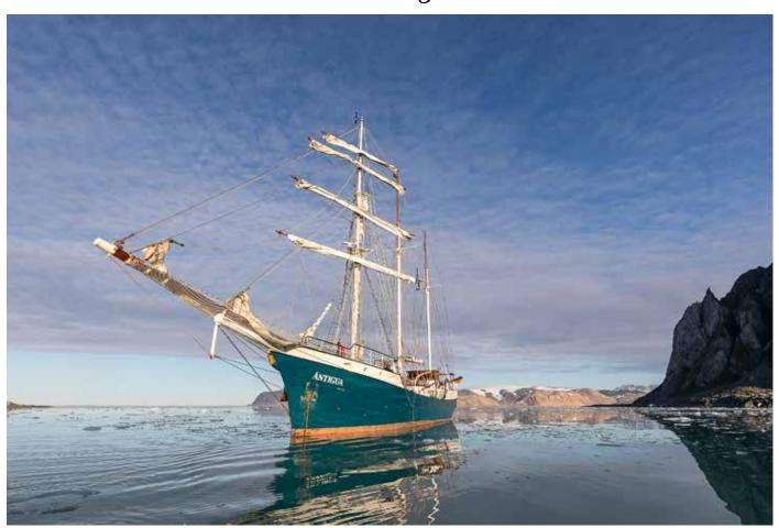
SV Antigua was built in 1957 in Thorne (UK) and served for many years as a fishing vessel, until it was completely rebuilt in the early 1990s in the Netherlands as a barkentine and equipped as a passenger ship. A barkentine has three masts with square sails on the foremast.
