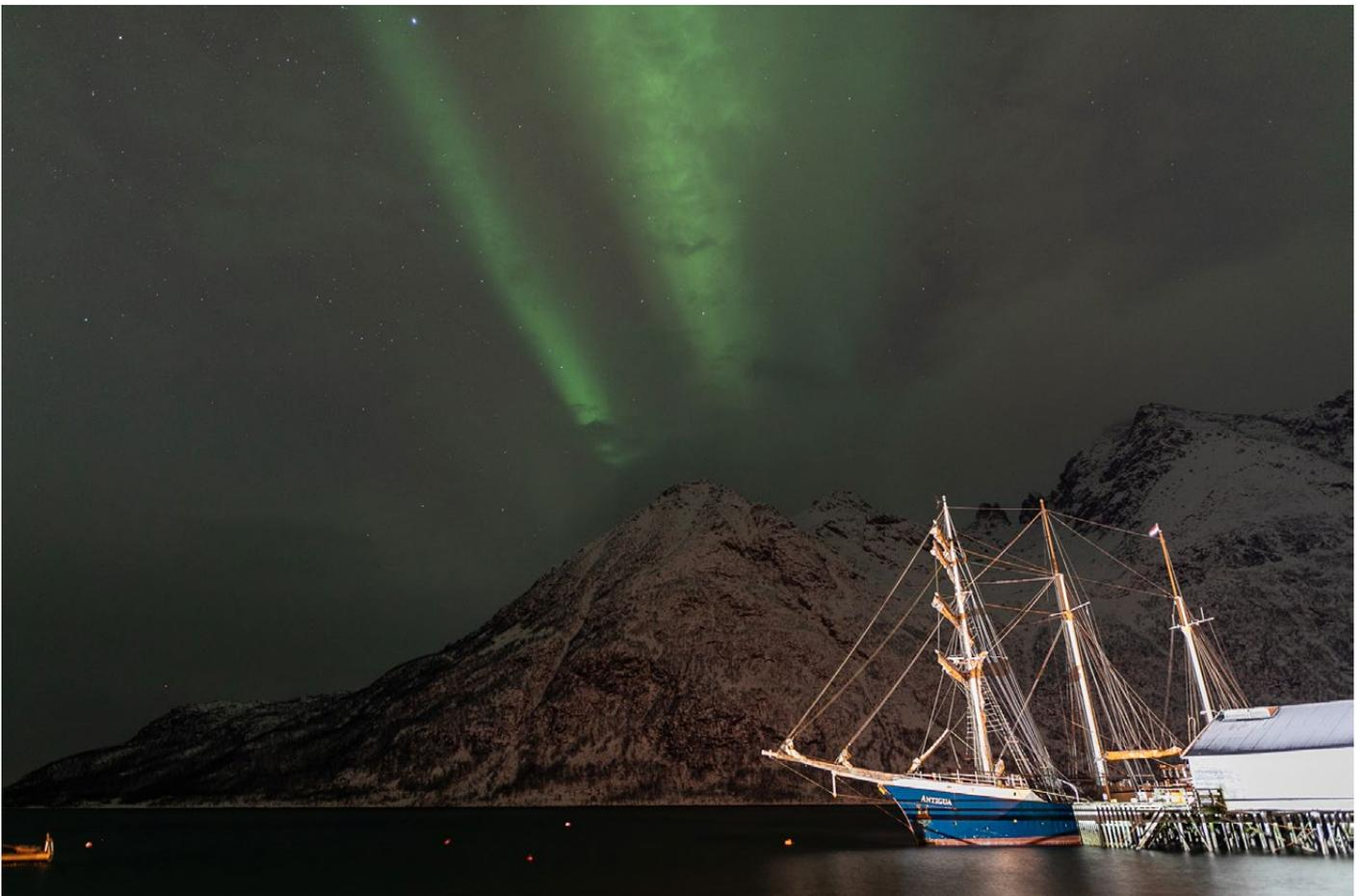
The SV *Antigua* was built in 1957 in Thorne (UK) and served for many years as a fishing vessel, until it was completely re-built in the early 1990s in the Netherlands as a barkentine and equipped as a passenger ship. A barkentine has three masts with square sails on the foremast.
